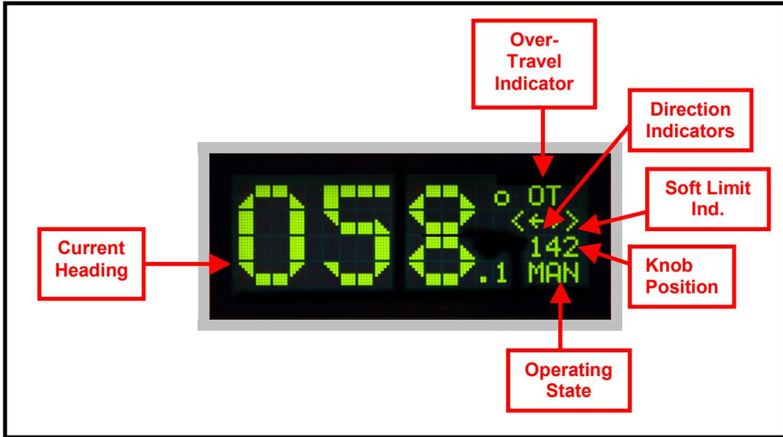
Figure 3. RT-20 Front Panel Display
