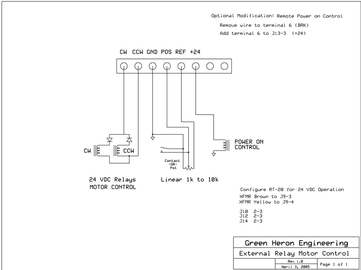
Figure C-1. External Relay Control
