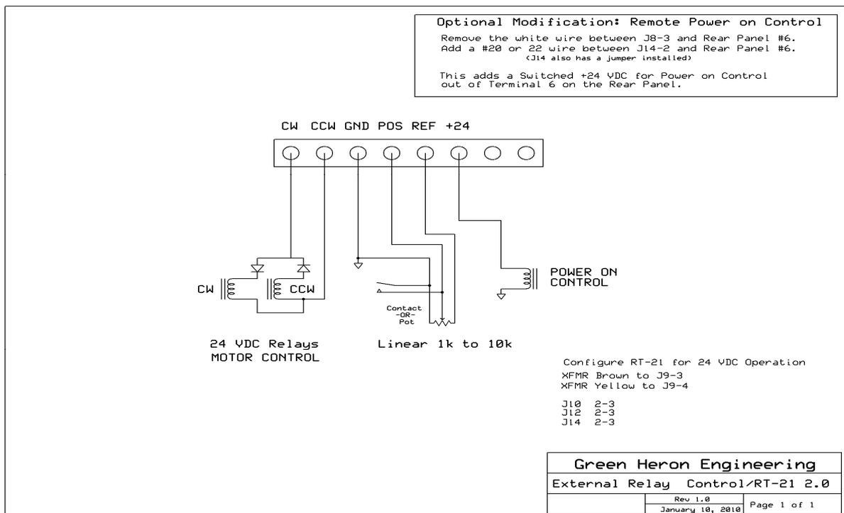
Figure C-1. External Relay Control
