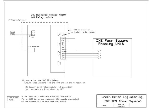
Create a WIO Profile using GHE Server Device Manger to create the on-screen display that you desire. Here's an example of a Map Display entry that uses the default compass rose for the background. This profile and wiring utilize the normal direction configuration of a 4 Square where NE is the default (all relays off) position.
